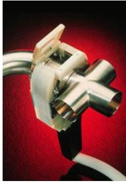
Figure 11 - Fittings Ready To Be Orbital Welded
