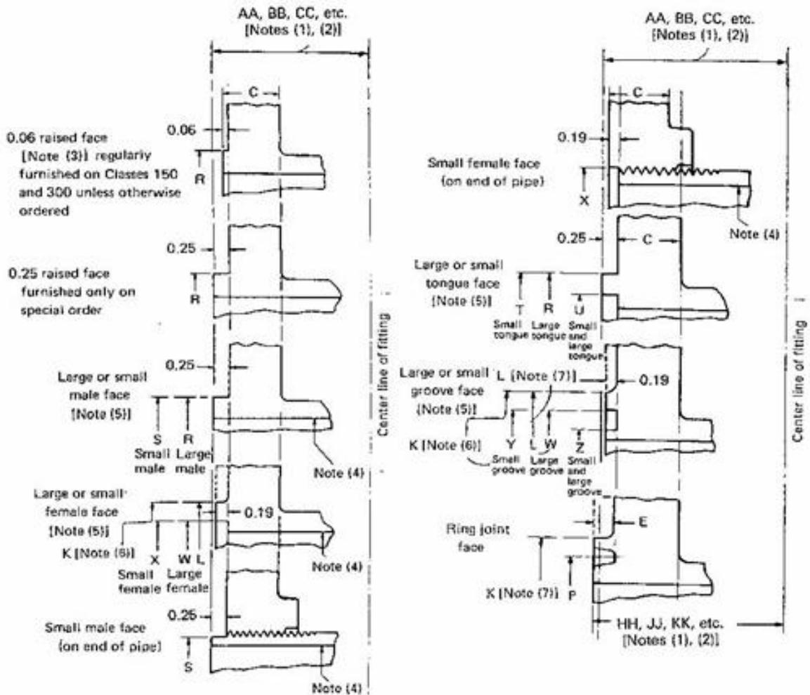
Figure 9 – Flange Facings from ASME B16.5
