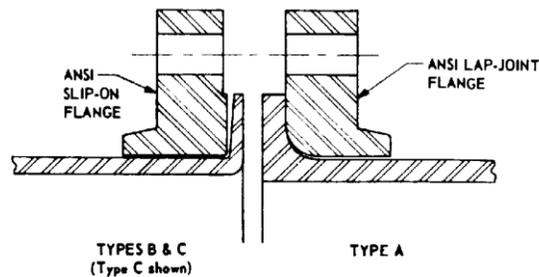
Type C (Fig 5) is fabricated from pipe using five suggested methods indicated in ASME B31.3. The most prevalent of these is the machine flare. This is done by placing a section of pipe into a flaring machine, flaring the end of the pipe and then cutting it to length.
