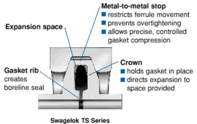
Figure 12 – Swagelok TS Series Profile
